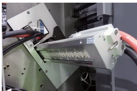
LED-UV curing unit in the delivery section
