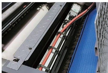
Inter-deck LED-UV curing unit over the impression cylinder
